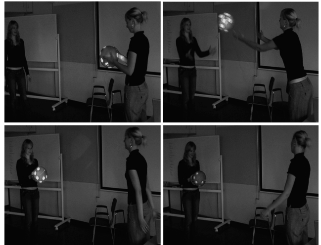
Figure 4: The Throw Ball light object targets the value Pleasure. This design is conceived for a person that likes to have fun in social setting. The final design is a ball the size of a soccer ball with holes in it that transmit light. The ball tries to stimulate people to throw it by blinking when it is held longer than 0.5 seconds. When it is thrown, it lights up fully. When held longer than 2 seconds, the light dies out which could mean the game is over.
