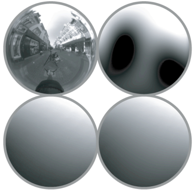
Figure 2 A panoramic image (a local light field measurement; upper left image) mapped on a sphere, which may be thought of as photographed on a specular sphere. The upper right image shows the superposition of the first three spherical harmonic components, which were shown separately in figure 1. The second row shows renderings of matte spheres in the high-resolution local light field and its low-pass approximation. It is clear that the superposition of flux density, light vector and squash tensor is sufficient to describe the appearance of such a matte convex object.
