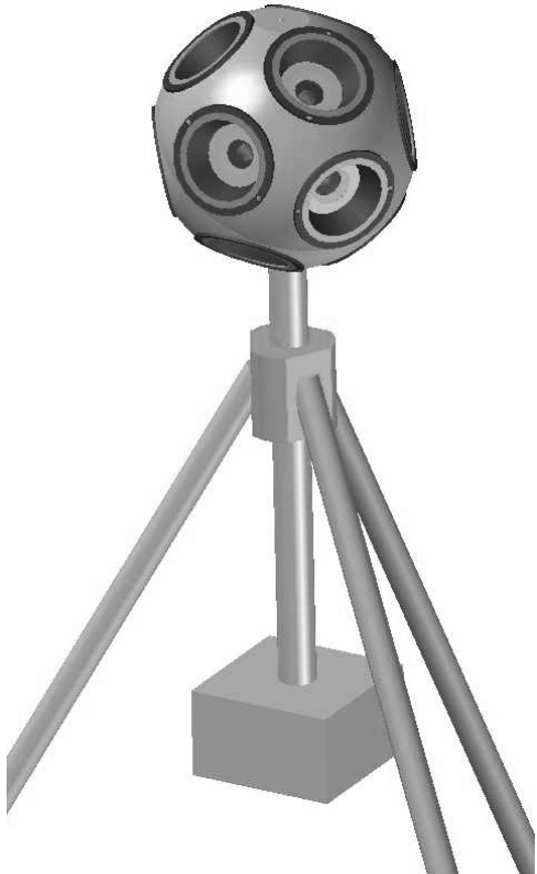
Figure 3 The plenopter: 12 high dynamic range sensors in a regular dodecahedron configuration. Local measurements result in 12 numbers from which we can estimate the second order spherical harmonic approximation. Sets of local measurements over an array of positions in 3D space allow for reconstructions of the light field in that space by interpolation.
